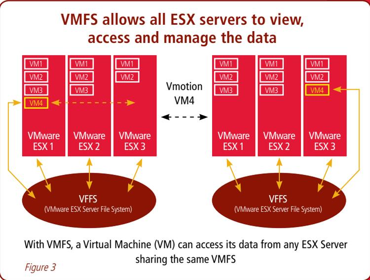
This high performance file system can span across the disks within a SAN (Fibre Channel or iSCSI) or on NAS appliances allowing all VMs access to their data regardless of which ESX server they are running on. It is also possible to directly attach a SAN LUN to a virtual machine (discussed later in the *Migrating from Physical to Virtual* section).
